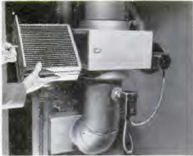
Heat-exchanger core is removed from Free Heater by simply releasing spring catch and pulling out drawer
